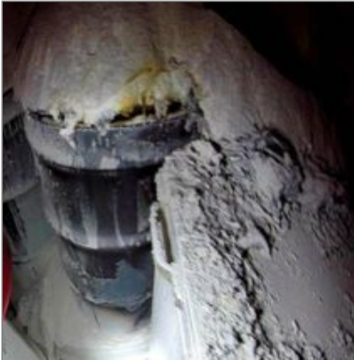
Figure 2-2. Visual evidence of breach of drum located at position 16-4 in P7R7 at WIPP
