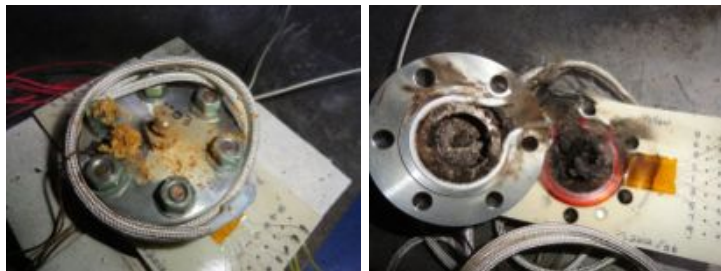
Figure G-26. Post-test images from Exp403. The left image shows that a substantial amount of material was expelled through the vent. The right image shows that the O-ring failed.
