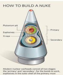
Modern nuclear warheads consist of two stages: the 'primary' and 'secondary'. For the bomb to work, explosives in the outer shell of the primary must detonate, squeezing a hollow sphere of nuclear material, usually plutonium-239, and triggering a runaway fission reaction. X-rays from the primary then cause atoms in the secondary's fuel to fuse and release still more energy.
