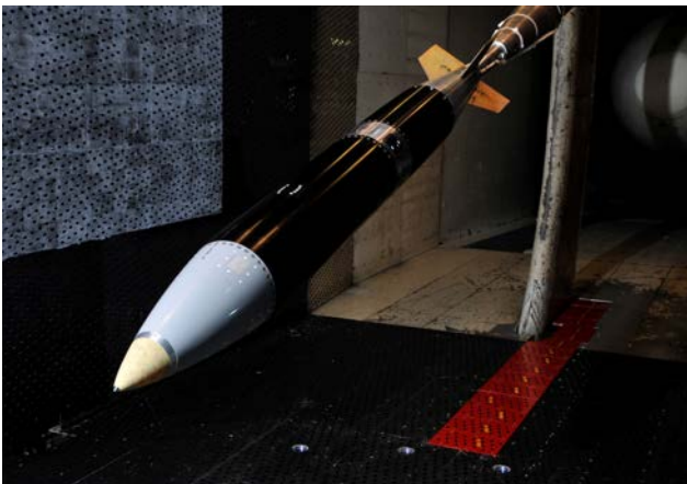
A B61-12 mounted on a wind tunnel test stand. The new guided tailfin kit is clearly visible, turning it into the world's first nuclear “smart” bomb.
