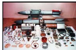
Components of 340 kiloton yield B61 gravity bomb.
