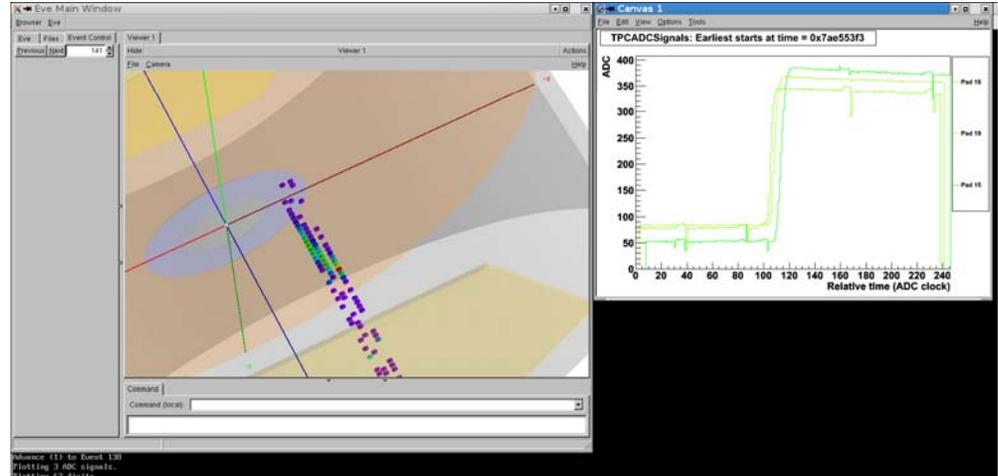
■ Track visualization of a single alpha decay. The software used for tracking and data analysis was specifically developed for the fission TPC.
