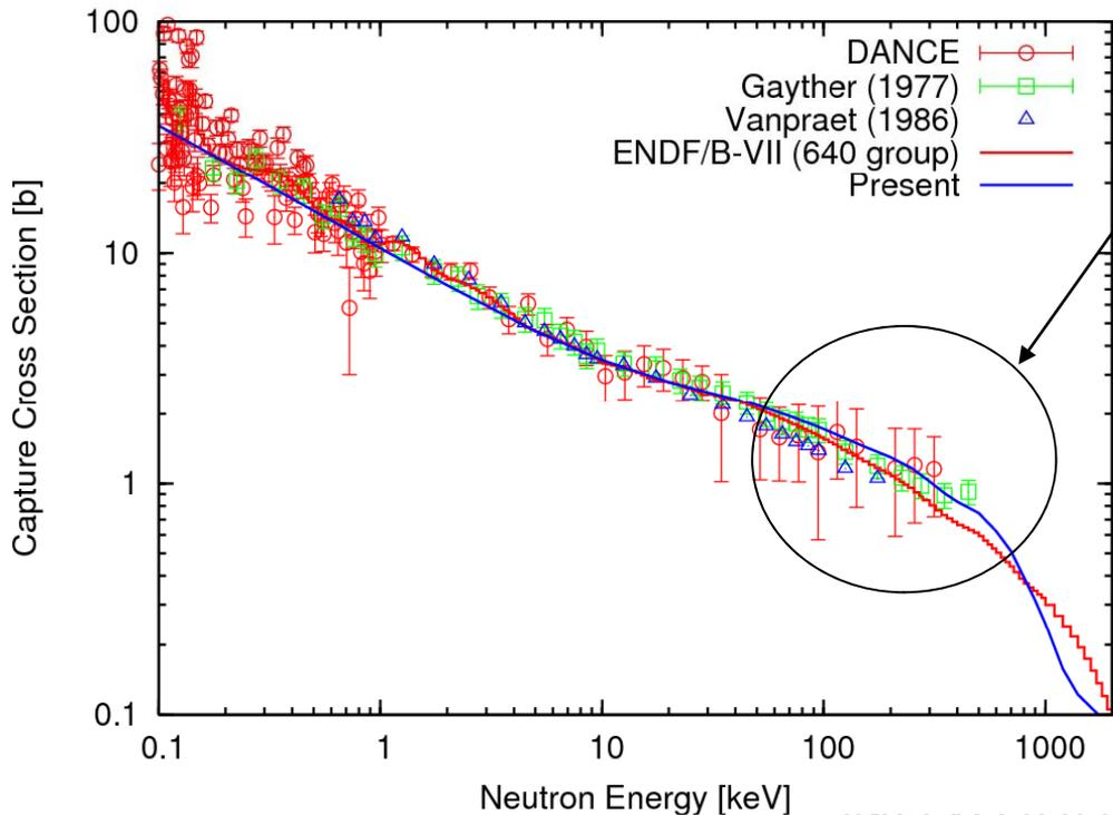
Critical assembly testing: when averaged over the Jezebel spectrum, gives 5% higher rate compared to ENDF/B-VII
