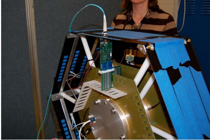
The fission TPC assembled with one complete electronic readout chain (32 channels). A Cm alpha source was used to produce signals in the first test.
