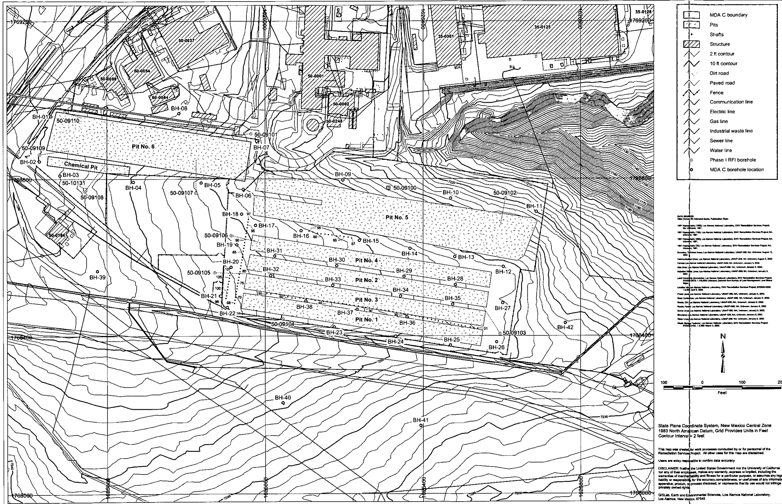
Figure 4.1-1. Location of proposed boreholes at MDA C
