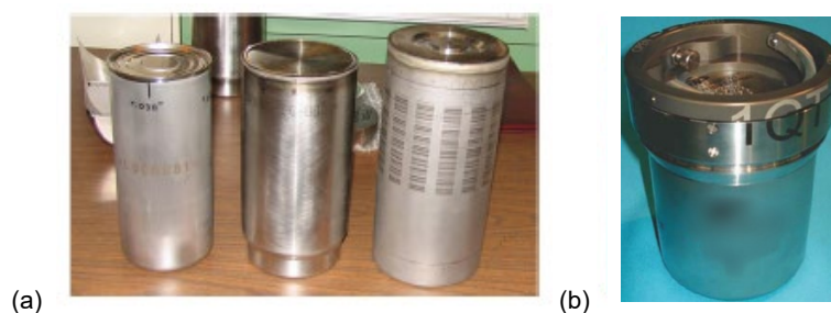
BOX FIGURE 1 The dilute and dispose program plan includes a transition from the 3013 containers: (a) nested cans of the 3013 container (left to right, convenience can, inner welded can, and outer welded can) to (b) a SAVY container. The SAVY container is a reusable container that has locking tabs and O-ring seals to eliminate welding. SOURCE: Cantey and Robertson, 2019. Images provided by the Department of Energy.
