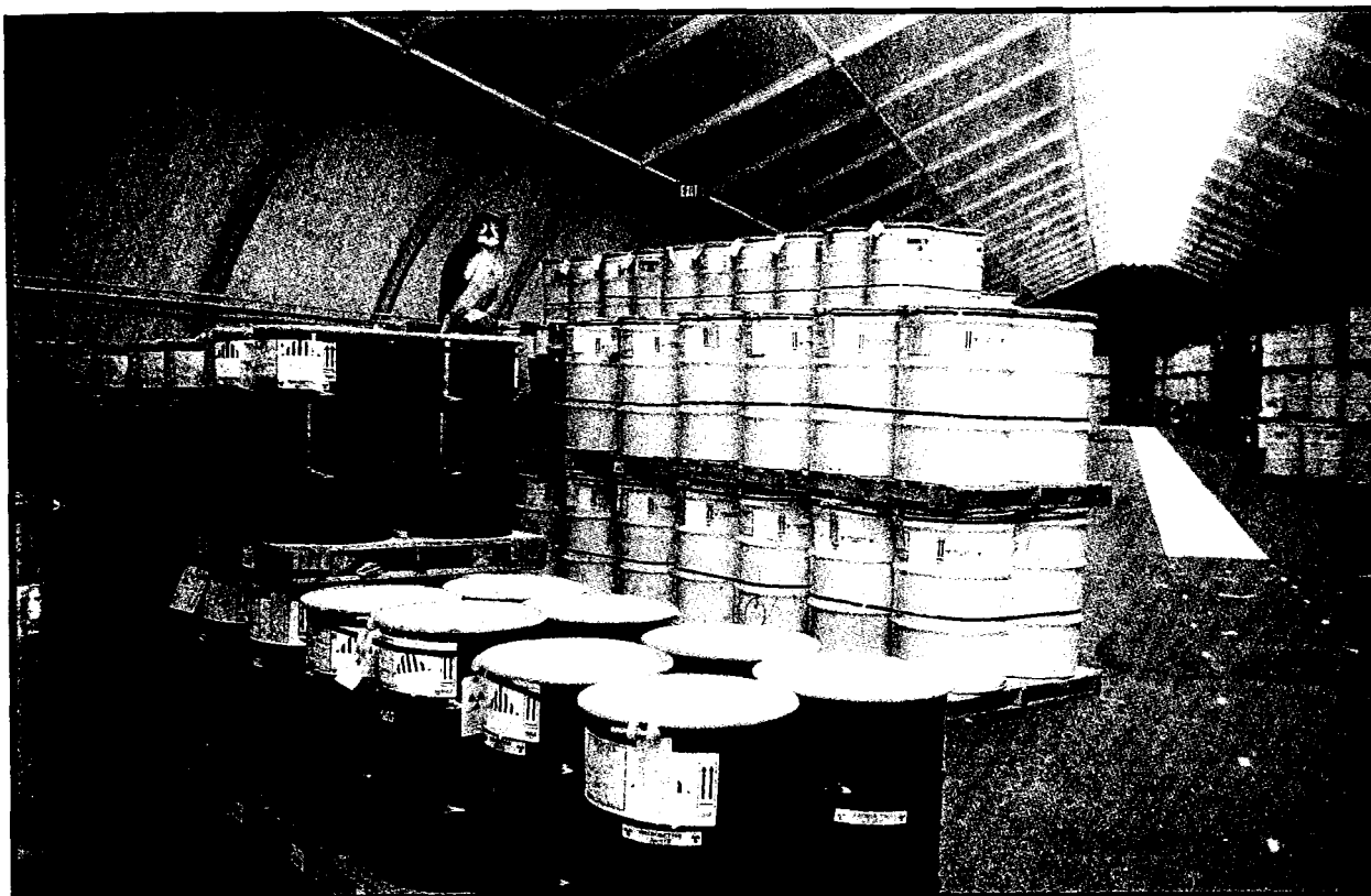
Waste. A painted plastic owl deters birds and mice from nesting among drums of transuranic waste inside a storage dome at the Los Alamos National Laboratory. The drums contain waste contaminated with plutonium and other long-lived radioactive heavy elements. Nuclear weapons research, design, and development generated most waste stored here. Transuranic Waste Storage Dome, Building 48 East, Technical Area 54, Area G, Los Alamos National Laboratory, New Mexico. February 24, 1994.
