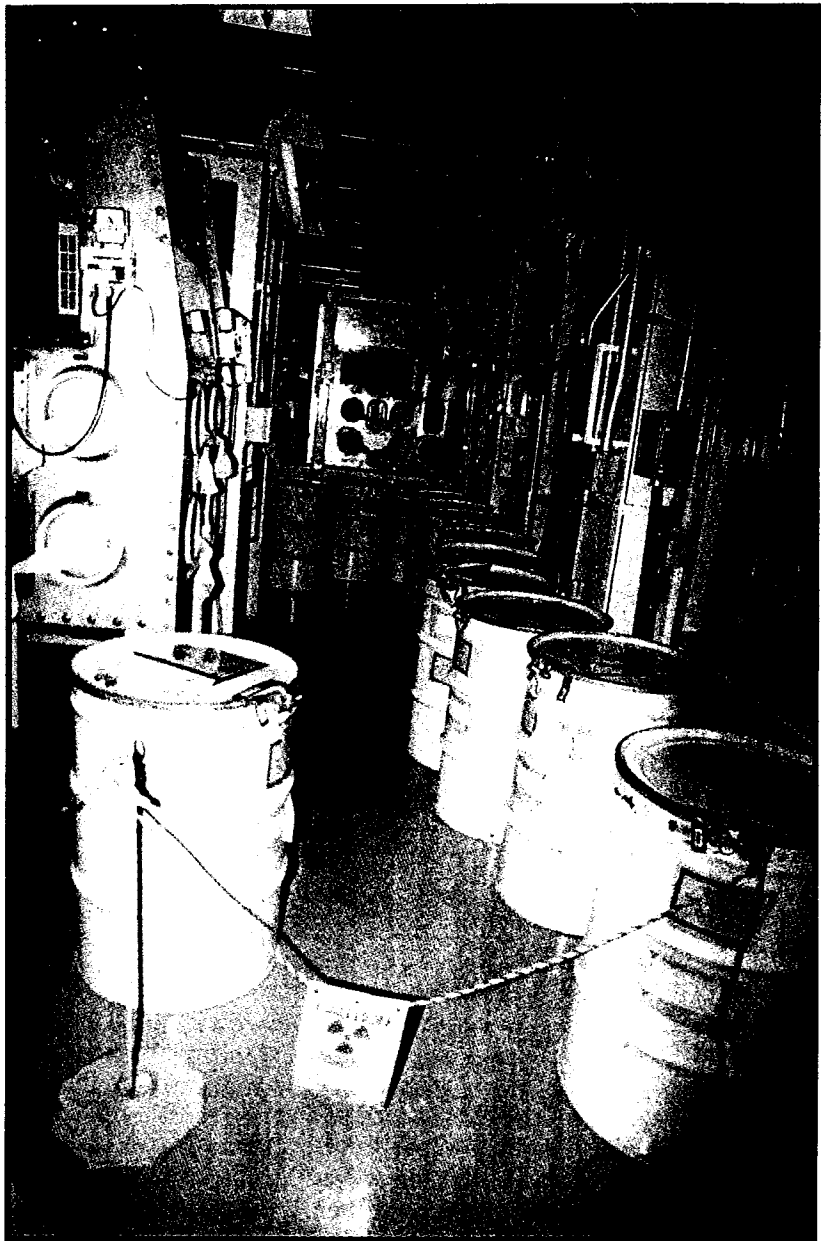
Drums of plutonium-bearing residues at the Rocky Flats Plant contain too much plutonium to be disposed of as transuranic wastes. The residues must be stabilized so that they can be stored safely until final disposition plans have been formulated and carried out. Building 776/777, Rocky Flats Plant, Colorado. December 20, 1993.
