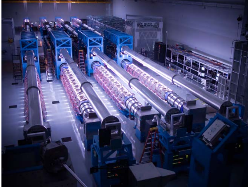
Figure A-5-4. A view of the OMEGA EP laser bay at the University of Rochester during a shot. The beamline structures are illuminated by a small amount of flash-lamp light that leaks out of the laser amplifiers.
