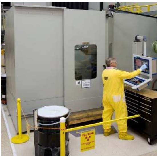
Figure A-1-6. Readiness Campaign achieved operational deployment of Multi-Axis Orbital Machining Center at Y-12 to support annual certification requirements.
