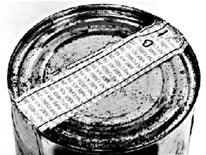
corroded "food pack" can containing plutonium, Hanford Nuclear Reservation
