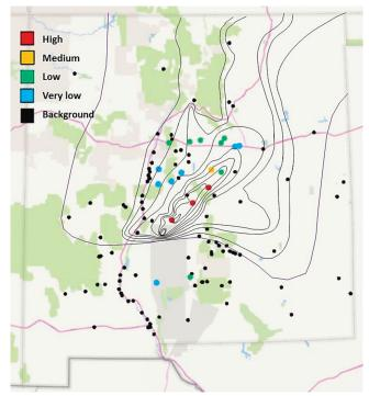
**Fig. 6.** Results of exposure measurements from Los Alamos Scientific Laboratory (Hoffman 1945) using x-ray film badges deployed in communities across the state before the Trinity detonation.
