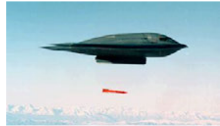
A B-2 drops a B61 Joint Test Assembly during a surveillance flight test.
