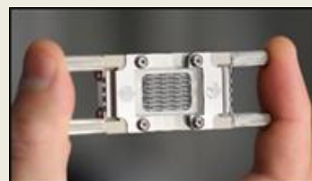
Micromixer chip for rapid mixing in the microreactor.
