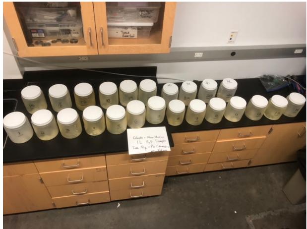
Water samples were evaporated in two liter polypropylene jars in a convection oven at at  $80-90^{\circ}$  C. The evaporated one liter water samples are shown prior to re-dissolution of the residue with 50 mL of 4 M HNO<sub>3</sub> (aq).
