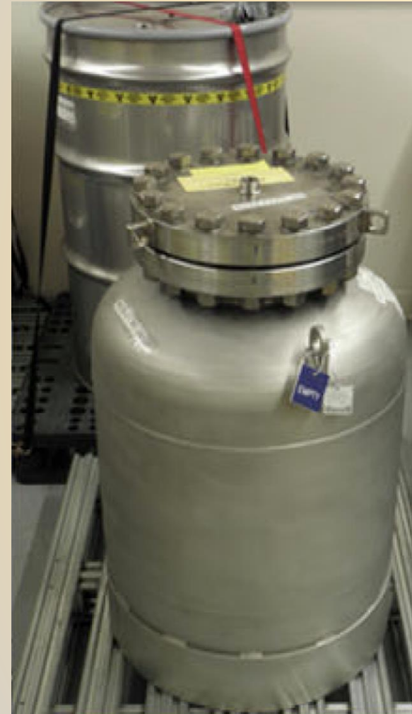
The FTWCs are approximately 50 gallons in size and are stored in 85-gallon steel drums.
